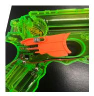
Above is the trigger (orange), the shell (green), and the electric circuit (starting from black below trigger going through the red and black wires).
