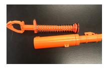
Above is the plunger (top), large spring (on plunger), and barrel (bottom) of the blaster. The air restrictor is in the barrel.
